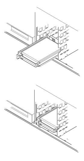
e. Move the carrier latch to the locked position. If the carrier does not lock, check that the drive carrier is fully seated in the backplane. When the drive carrier is fully seated, the green LED on the drive carrier illuminates.
